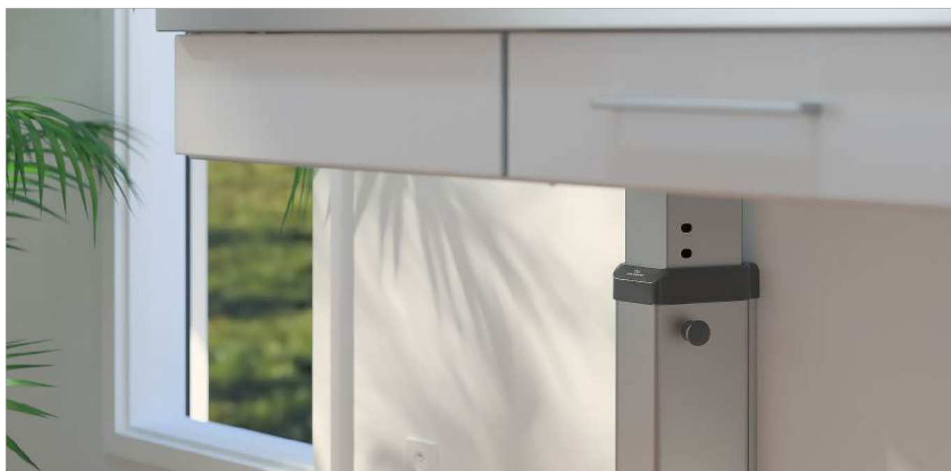
A built-in gas spring facilitates height adjustment: Pull out the locking pin, adjust the height, (the gas spring provides lifting help). Lock the position with the locking pin.
